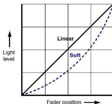
**Figure 2. Dimming curves**
