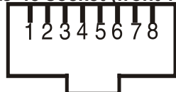
RJ-45 socket (front view):
