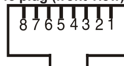
RJ-45 plug (front view):
