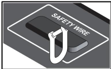
Fasten a safety cable (not shown) between the support structure and the attachment point on the fixture. The safety cable must be able to bear at least 10 times the weight of the fixture.
