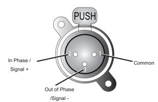
**NOTE:** This pinout is for a balanced input. For unbalanced input, make the following connections in the user cable: Connect XLR pin 1 and pin 3 together, tying Common to Signal -. The unbalanced signal connects to XLR pin 2, Signal +.
