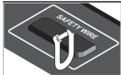
Fasten a safety cable (not shown) between the support structure and the attachment point on the fixture. The safety cable must be able to bear at least 10 times the weight of the fixture.
